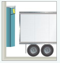
Vehicle approaches WeatherGuard Header Seal while being positioned at the dock door opening.
