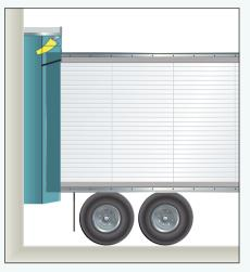
When vehicle is in position at the dock, the helical torsion springs of the pivoting head member provides consistent tension force over the width of the unit while ensuring the foam head member conforms to the top of the trailer creating a watertight wiper seal.
