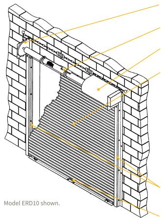
**BRACKETS** - Steel with powder coating to match curtain. Bolt to guide assembly and support counter-balance shaft curtain.
