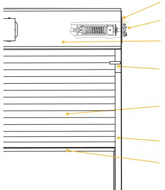
**BRACKETS** - Steel with powder coating to match curtain. Bolt to guide assembly and support counter-balance shaft and curtain.
