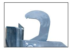
Rotating Steel Hook: The deeper hook profile increases the size of rear impact bars (RIG) that can be engaged. The hook shape reduces the stresses on the restraint as well as the RIG by spreading the stresses more evenly.
