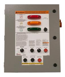
Combination control panels combine the controls for loading dock equipment such as vehicle restraint system, hydraulic dock leveler, overhead door and inflatable dock shelter into a single common panel. This ensures proper use and sequencing of equipment for increased safety and ease of operation.
